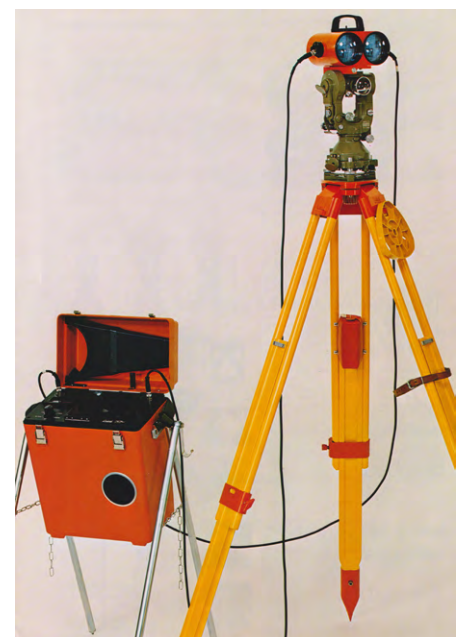
Fig. 9: The DISTOMAT DI10 on a T2 theodolite together with the control unit.
