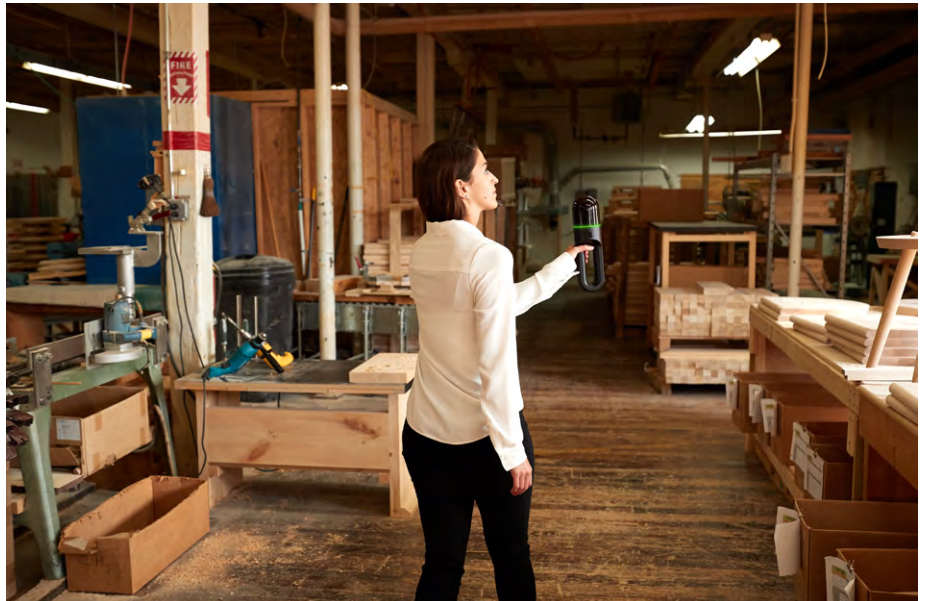
Fig. 17: The BLK2GO hand-held laser-imaging scanner digitises space in 3D while you move.
