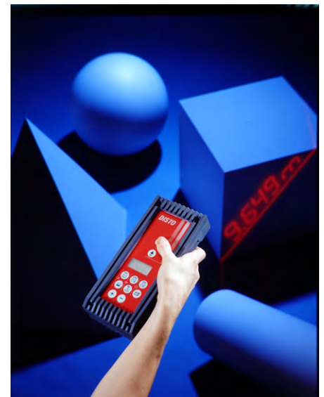
Fig. 15: The original DISTO of 1993 – still weighing 900 g and rather expensive.
