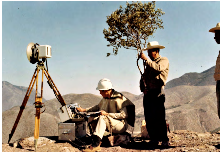
Fig. 8: To measure a distance between 100 m and 50 km, a DI50 was set up at each end-point and the distance calculated by measuring the transit time of the microwave radiation. The picture shows a DI50 being used in Mexico.
